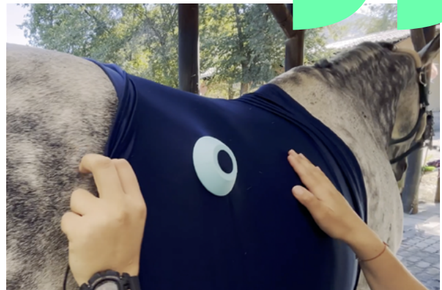
01. Device for capture, monitoring and biometric analysis of bowel sounds
